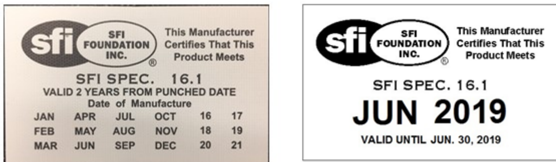
Figure B-31: Driver Harness, SFI Tag, Old Style (Left), New Style (Right)
