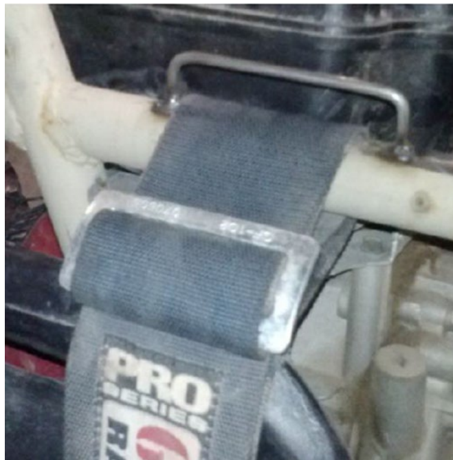
Figure B-34: Driver Harness, Shoulder Harness Lateral Restraint
